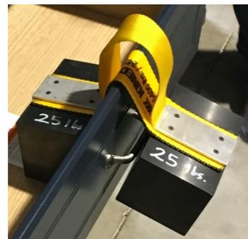
The 50-pound weight used in the *Stability with Load Test*
